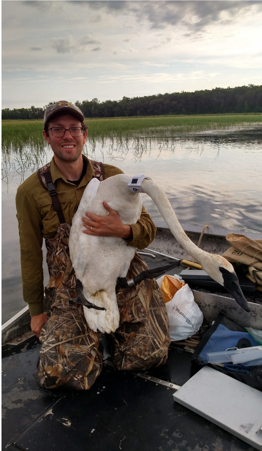
Figure 2. An example of the Ornitela OrniTrack-N62 collars with GPS/GSM transmitter incorporated into the internal housing that were deployed in Minnesota during 2019. All new deployments in 2020 will be this design.
